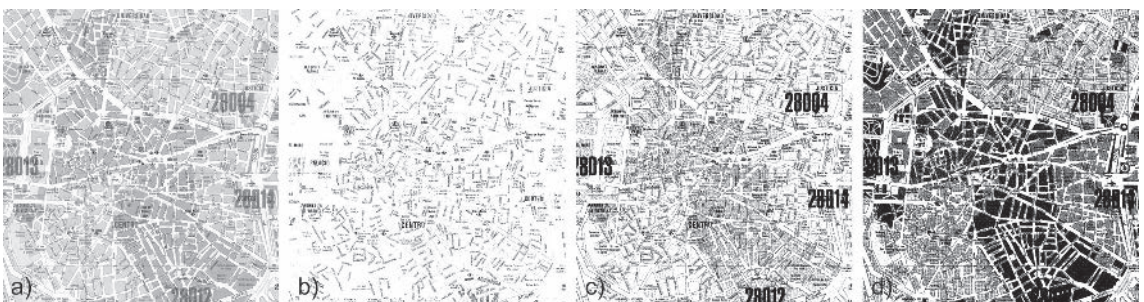
Fig. 2. Binarization of city map: a) digitized fragment; b), c) and d) images after binarization with thresholds 128, 180 and 220 DN, respectively
