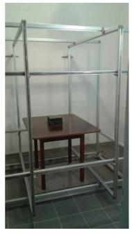
Fig. 3. The coil developed in the Central Geophysical Observatory of the Institute of Geophysics of the Polish Academy of Sciences in Belsk used to check the proton magnetometer
