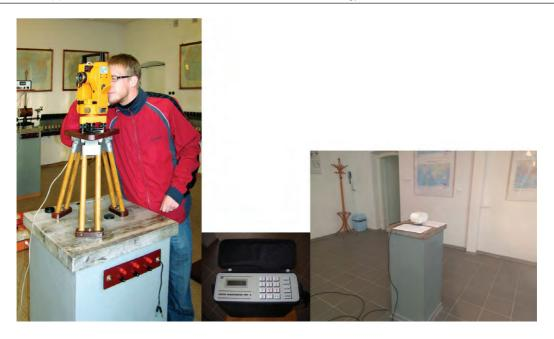
Fig. 5. The measurement of magnetic declination, inclination and module *F* of the total intensity vector on the base pillar in Belsk observatory
