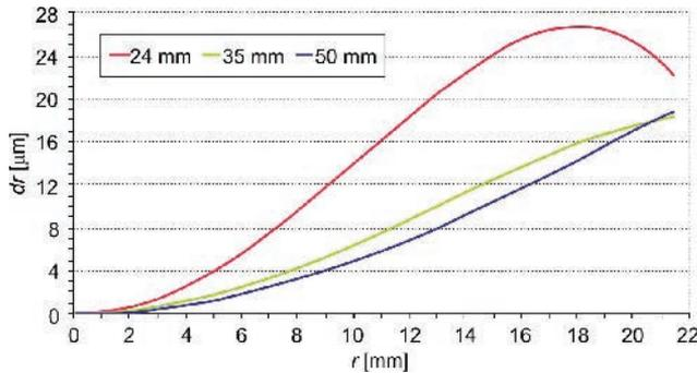
Fig. 4. Radial distortion of tested lenses obtained from the calibration using 3D test field
