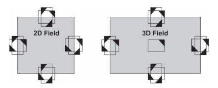
Fig. 3. Images configurations for calibration in PhotoModeler for 2D field (left) and 3D field (right)
