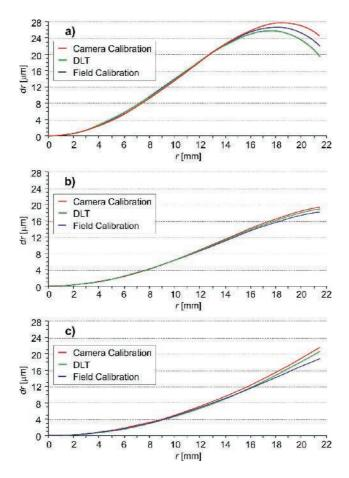
Fig. 5. Radial distortion of 25 mm lens a), 35 mm lens b) and 50 mm lens c) for three calibration methods applied
