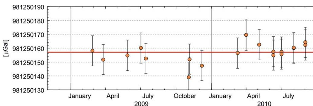
Fig. 2. Results of measurements with the A10-020 at the field station 156 Borowa Gora.
