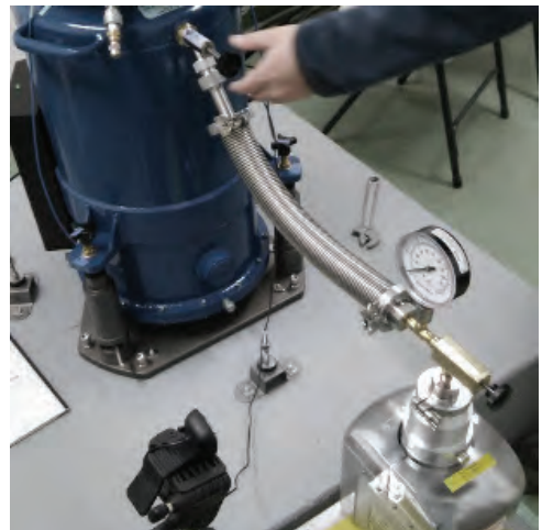
Fig. 7. Pumping the dewar vacuum insulation
