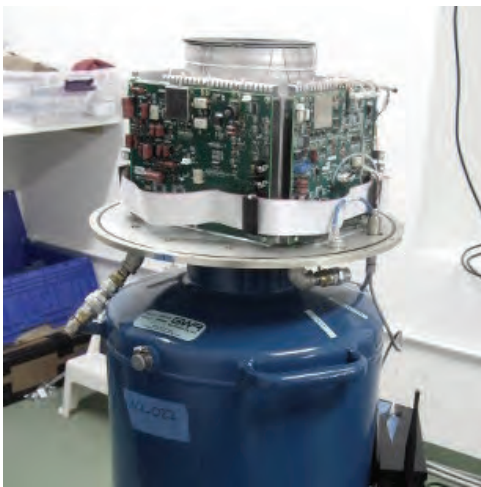
Fig. 4. Removal of the dewar head cover
