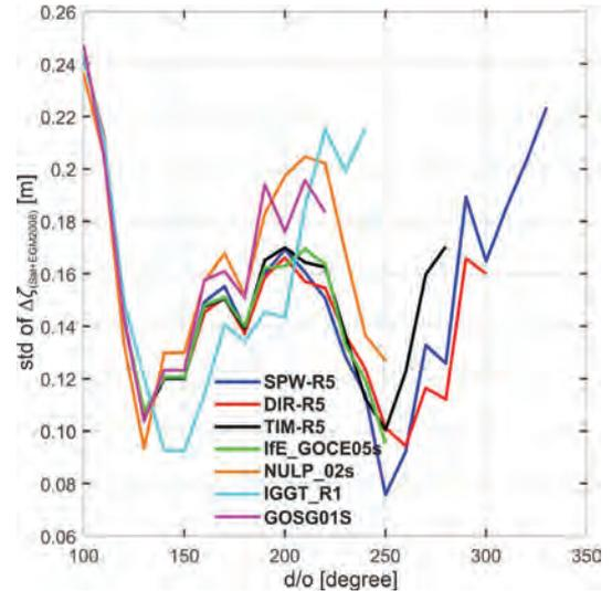
Fig. 6. Standard deviations of differences  $\Delta\zeta_{(Sat+EGM2008)}$  for Uganda
