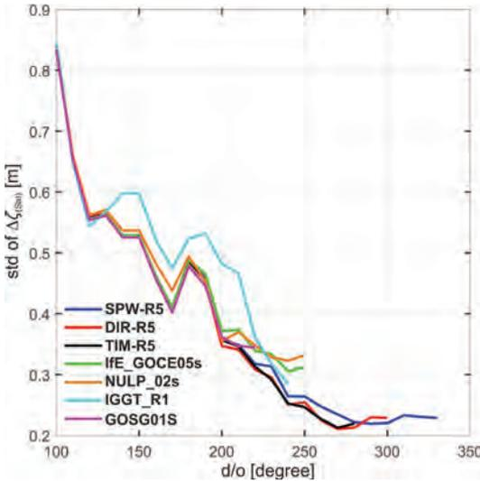
Fig. 5. Standard deviations of differences  $\Delta\zeta_{(Sat)}$  for Uganda
